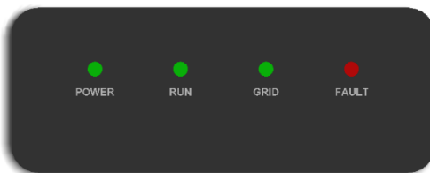
Figure 7-1 LED display of the inverter Indicators and their indications are shown in Table 7-1.
