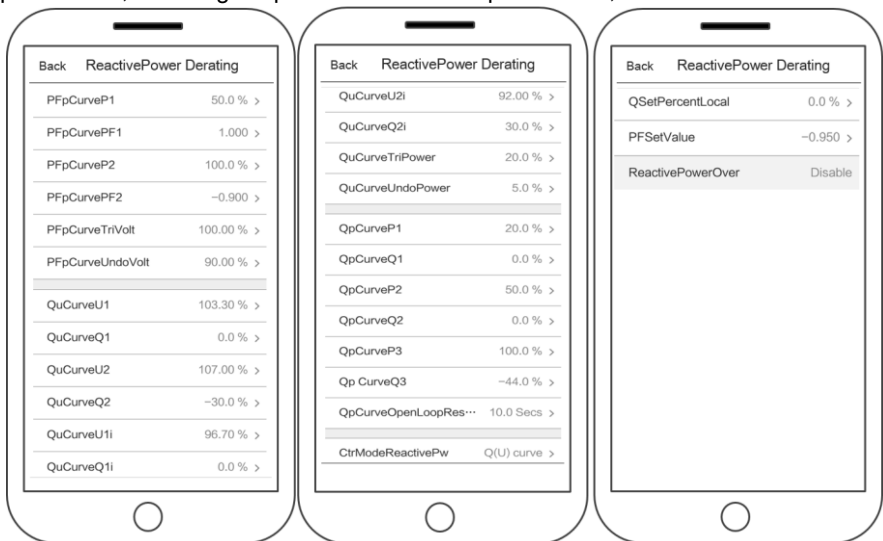
Figure 6-16 The ReactivePowerDerating interface
