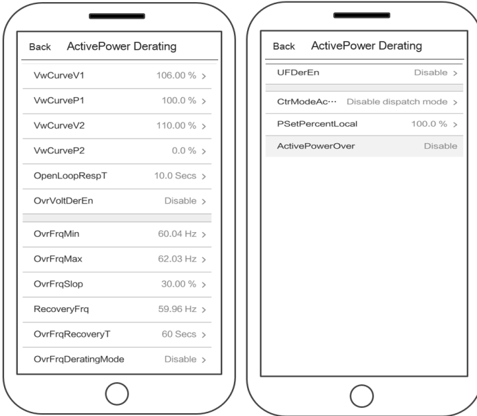
Figure 6-13 ActivePower Derating interface
