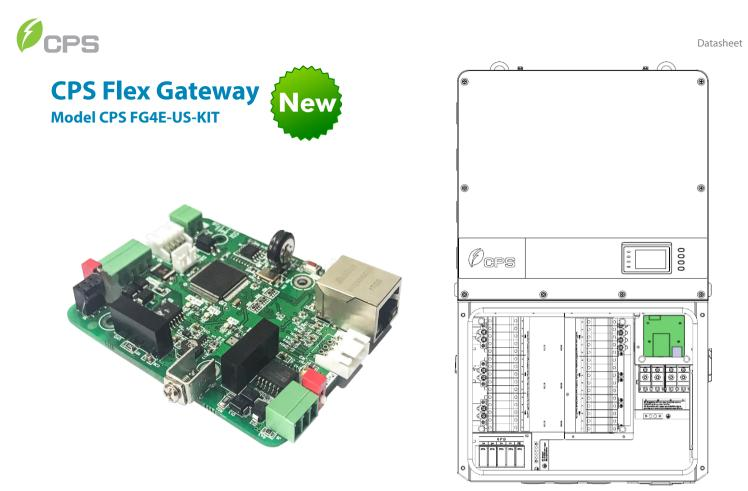
The CPS Flex Gateway is a new communications and controls solution for the CPS 36, 50, 60, 100 and 125kW inverters. The gateway is a Modbus master data logger and communications device. This flexible solution enables three parallel outbound communication options: (1) local pass-through Modbus RS485 data to 3rd party solutions, (2) Ethernet based communications for CPS service operations, and (3) a programmable Ethernet based connection to a location chosen by the customer.
