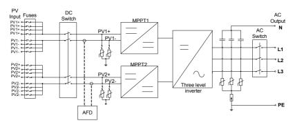
Figure 2-2 Schematic diagram of CPS SCA36KTL-DO/US inverter
