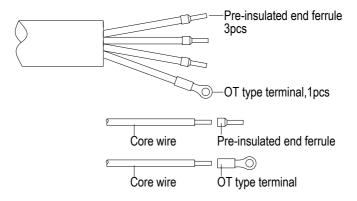
Figure 3-29 AC output and ground cable set up
