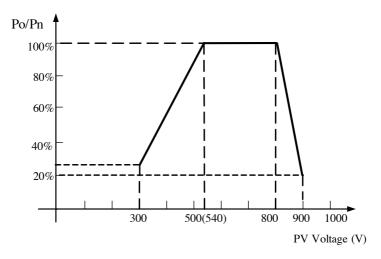
Figure 8-1 SCA36KTL derating curve of PV input voltage
