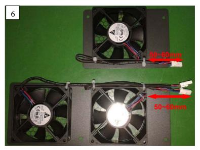
Figure 7-1 Replace cooling fans
