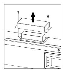
Figure 3-10 Cover board of the wiring box
