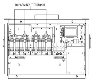
Figure A-1 Internal structure of CPS SCA36KTL-DO inverter with optional components
