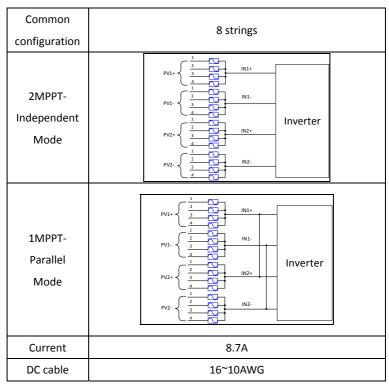
Note 1: The temperature rating of the input wirings should be no less than  $90^{\circ}\text{C}(194^{\circ}\text{F})$ .
