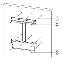
Figure 3-6 Secure the mounting bracket
