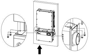
Figure 3-11 Installation of the wiring box
