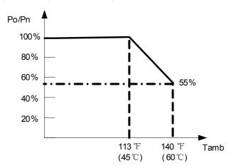
Figure 8-2 SCA36KTL derating curve with high temperature
