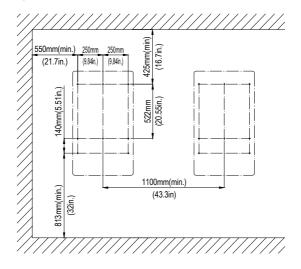
Figure 3-5 Dimensions of holes on the bearing surface
