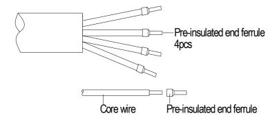
Figure 3-28 AC output and ground cable set up
