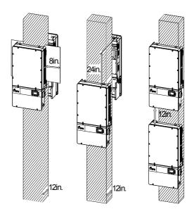
Figure 3-4 Inverter pillar mounting dimensions
