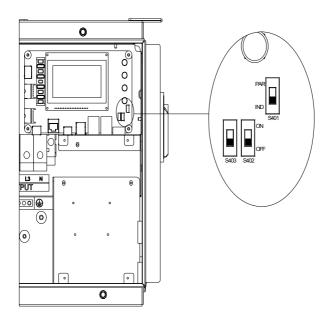
Figure 3-22 Location of the PV connection mode selector switch
