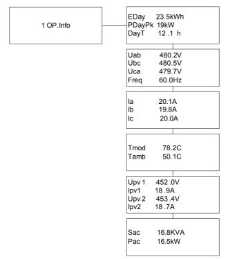
Figure 5-8 Operation information indication (PV independent mode)
