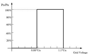
Figure 8-4 SCA36KTL derating curve of grid voltage
