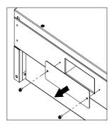
Figure 3-9 Cover plate of the main housing
