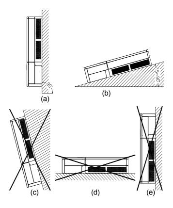
Figure 3-2 Mount the inverter correctly
