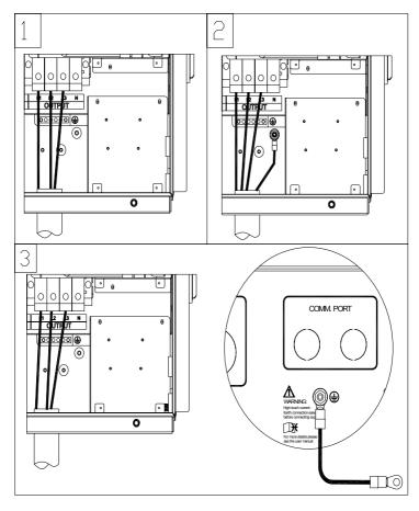
Figure 3-27(a) AC output and ground cable connection
