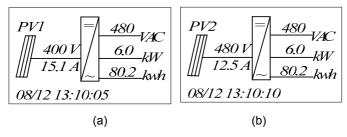
Figure 6-2 Default indication interface for normal operation
