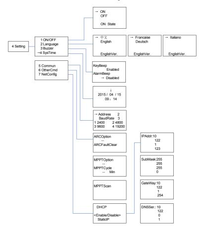
Figure 5-12 System setup menu and submenu
