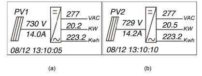
Figure 5-5 Default display interface for normal operation
