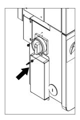
Figure 3-13 Attach the cover board to the left side of the wiring box
