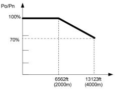
Figure 8-3 SCA36KTL derating curve with high altitude
