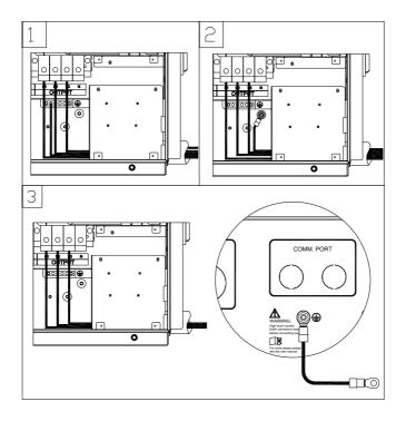
Figure 3-27(b) AC output and ground cable connection
