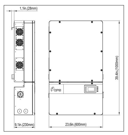
Figure 3-1 Dimensions of CPS SCA36KTL-DO/US inverter
