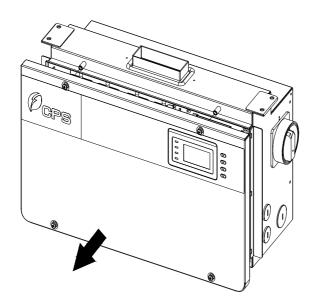
Figure 3-26 Take off the cover of the wiring box
