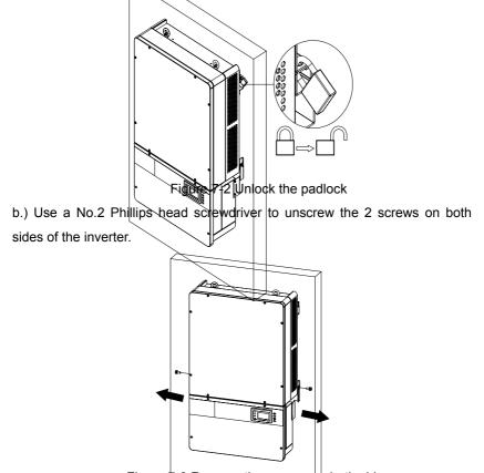
Figure 7-3 Remove the screws on both sides
