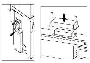
Figure 7-5 Install the cover board on the connector of the wiring box
