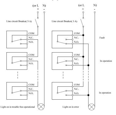
Figure 3-33 Schematic diagram of dry contact communication
