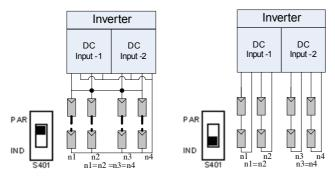
Figure 3-20(a) Parallel mode Figure 3-20(b) Independent mode
