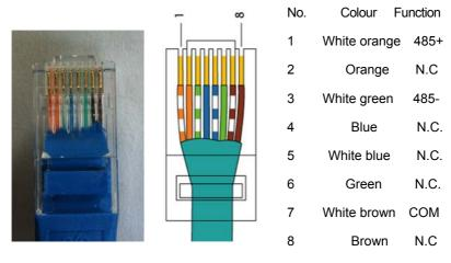
Figure 3-38 Crimp RJ45 connector on the RS485 and Ethernet cable
