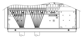
Figure 3-25(a) Connection of DC input cables
