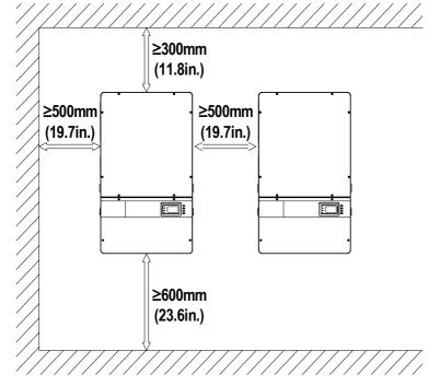
Figure 3-3 Inverter wall mounting dimensions
