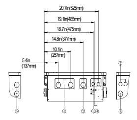
Figure 3-18 External connection ports
