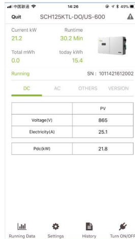
Figure 4-3 Normal Operation Status
