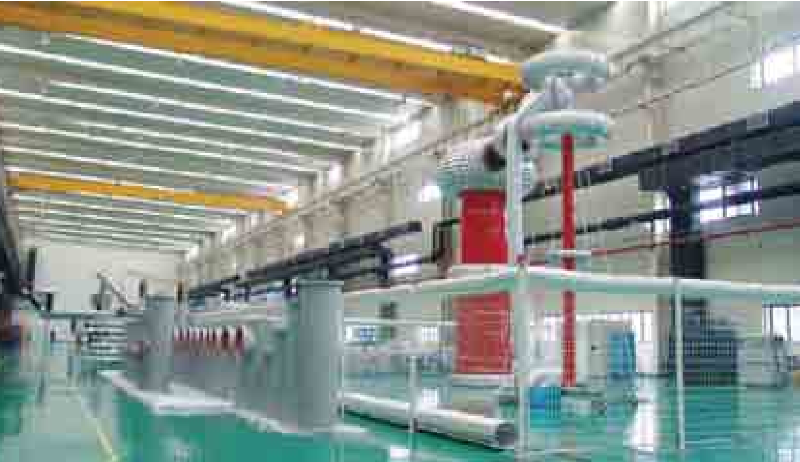
750kV Power frequency withstand voltage test transformer
